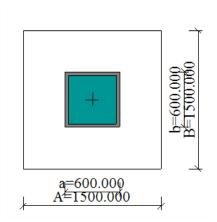
B' = min (L1 ; L2) L' = max (L1 ; L2) A' = B' \* L'
