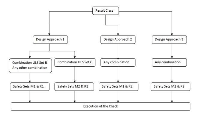
• For **Design Approach 1** the safety sets depend on the combination type. For combinations of type **EN-ULS (STR/GEO) Set B** sets **M1** & **R1** are used.
