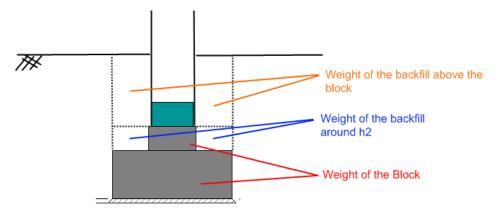
The design value of the total weight G can then be calculated as follows:
