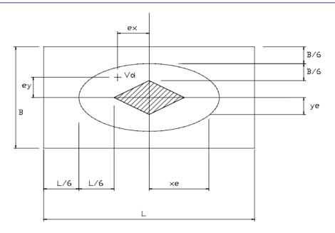
The eccentricity check of **1/6** take into account that the whole pad foundation is under pressure. The foundation will not lose contact with the ground over the whole area.
