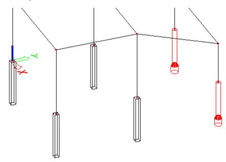
The colour of the Pile is from the Pile plan library. The colour of piles is controlled by the view flag parameters under the tab "Model"
