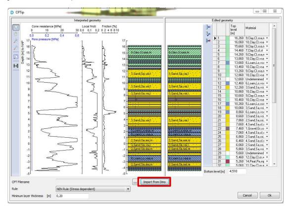
The program generates the soil profile from the CPT data. In this dialog, two soil profiles are drawn. The left profile is the result of the interpretation from the CPT data with the CPT data drawn to the left of it and the other profile is the edited geometry.
